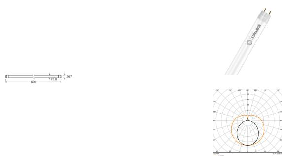
**Scheda tecnica Ledvance Tubo LED T8 EM Superior Conventional (EM), Mains (AC) High Output T8 6.3W 1100lm - 865 Luce Del Giorno | 60cm - Sostitutiva 18W**
